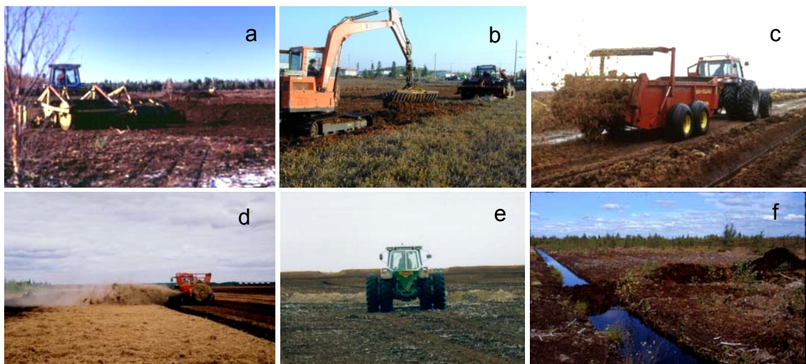
Figure 8: The six main mechanical steps for the Canadian approach to restore milled harvested peatlands. (Photos taken by Peatland Ecology Research Group).
