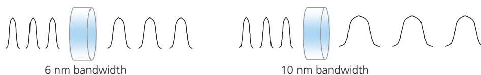
Fig. 8-7 Effect of GVD on short pulses with a broad bandwidth. The broader the bandwidth, the more the pulse is stretched. Longer wavelengths travel faster through the glass than shorter wavelengths in the pulse. Thus, a positively chirped pulse is broadened.
