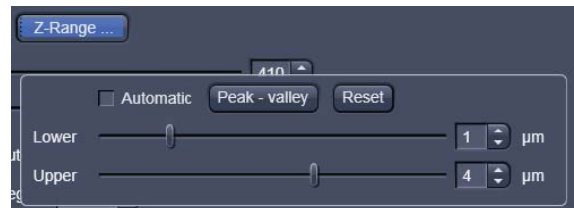
Fig. 4-214 Z-Range pop up to define height thresholds
