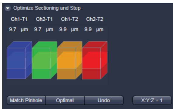
Fig. 4-60 Optimize Sectioning and Step: Match Pinhole to Step resulting in equal optical sections for all channels
