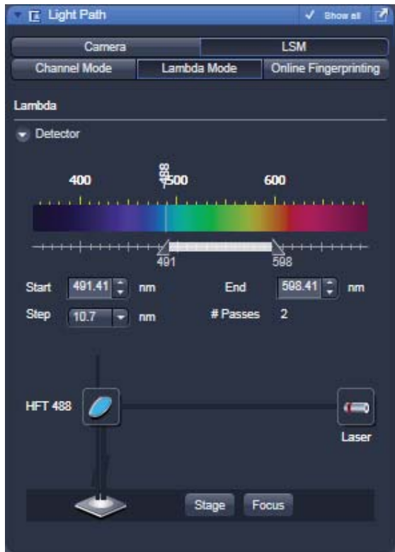
Fig. 4-43 Light Path tool window; Lambda Mode activated
