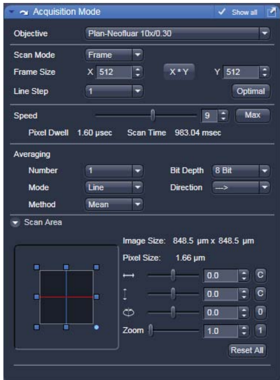
Fig. 4-46 Acquisition Mode - Frame with LSM tab selected in the Light Path tool
