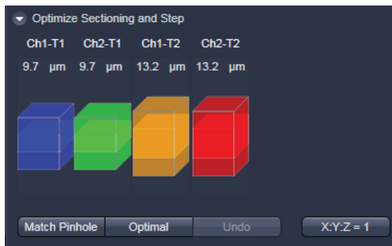
Fig. 4-59 Optimize Sectioning and Step: Optimal Interval is set starting with one Airy unit for all channels
