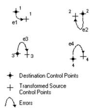
Take the root mean square (**RMS**) sum of all the residuals to compute the total RMS error; this value describes how consistent the transformation is between different control points.
