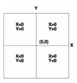
In a **projected** coordinate system, a twodimensional flat surface defines locations based on a geographic coordinate system as x,y coordinates identified on a grid. Unlike a geographic coordinate system, a projected coordinate system has constant lengths, angles, and areas across the two dimensions. In a projected coordinate system, locations are identified as follows:
