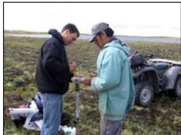
Andrew Medeiros and Andy Aliyak extruding a sediment core, July 21, 2006. (photo by A. Namayandeh)
